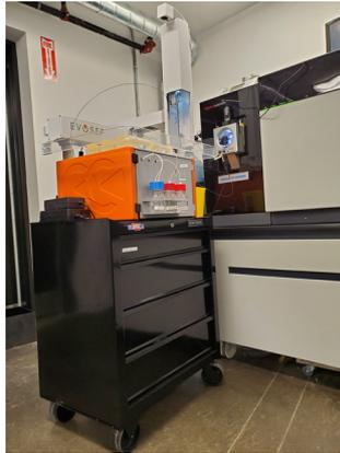
**Figure 2:** A fleet of eight Evosep Ones are shuttled and connected to mass spectrometers that run 24/7, creating a continuous production line of proteomic data. “We were going to name our Evosep Ones after the Seven Dwarfs,” says Paul Taylor, Core Facility Manager. “But now we have eight of them.”
