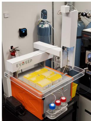
**Figure 1:** An Evosep One connected to a mass spectrometer at Rapid Novor. To enable continuous data production, the Rapid Novor team uses cameras to remotely monitor each Evosep One as it moves samples through Evotips and onto the liquid chromatography column.
