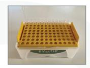
Place the Evotips in the centrifuge with appropriate counter balance and centrifuge at 800 g for 60 seconds.
