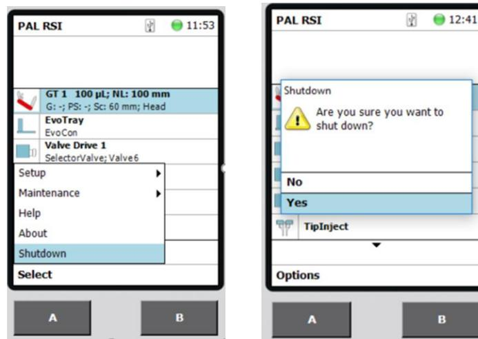
5. When the terminal window turns off, switch off the power on the autosampler power supply and wait for the Z-axis to drop into lock position.
