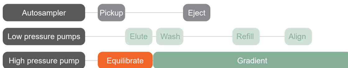
Figure 2: The steps between injections are performed in parallel to reduce overhead time.
