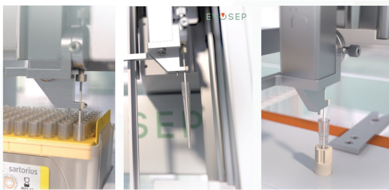
Figure 1. Upon starting an analysis, the autosampler places one tip at the time (with the pre-loaded sample) in-line with the solvent system
