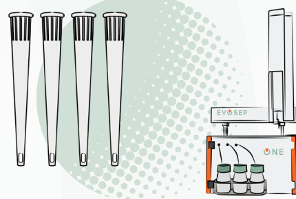
Figure 1: Evotip Pure integrates peptide purification with sample loading and elution.
