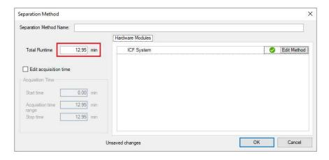
5. Give the Separation Method the same name as chosen in the ICF System Method Dialog, e.g. "100 samples per day" and click "OK".
