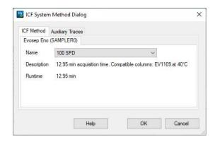
4. Now check/set the Total Runtime for the chosen method using below table and/or Runtime from above dialog. Below example is given for the 100 samples per day method.
