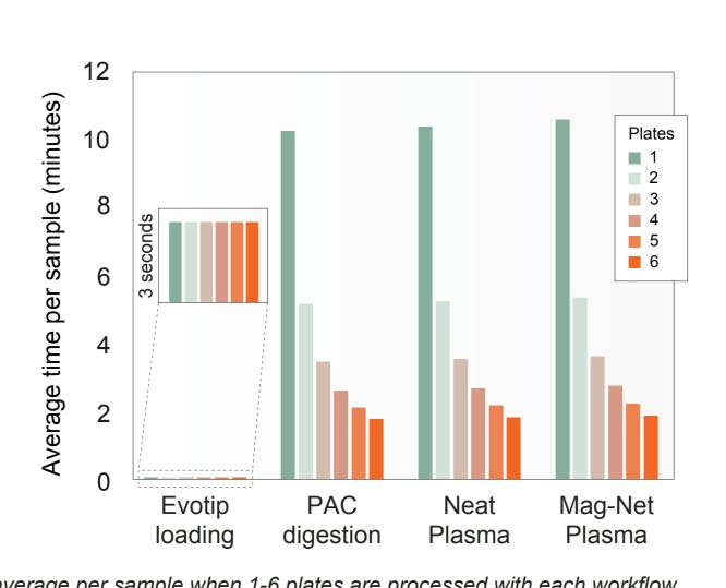
Schematic representation of deck layout on the Biomek i5 and an overview of how much time on is spent on average per sample when 1-6 plates are processed with each workflow.
