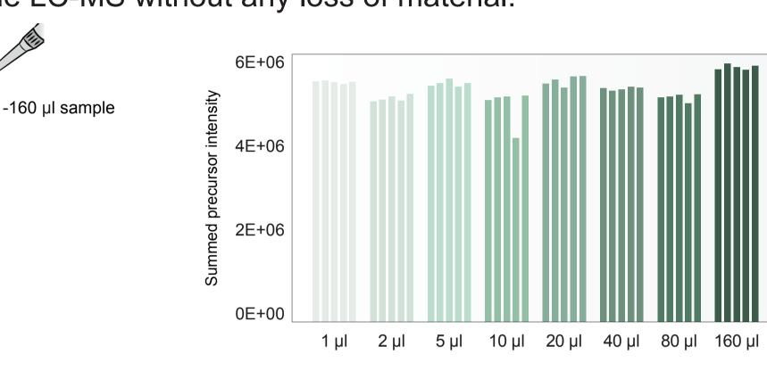
Summed precursor intensities of 250 pg HeLa loaded on Evotips in 1-160 µl solvent A. Evotips loaded with volumes lower than 20 µl had solvent A already deposited in them for a total loading volume of 20 µl. Samples were analyzed with Whisper 40 SPD.
