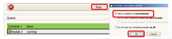
Make sure that the sequence is also removed from the Xcalibur queue, or it may block subsequent jobs.
