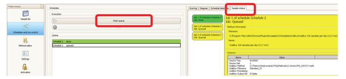
f. Open the MS data acquisition program and verify that MS is waiting for contact closure.
